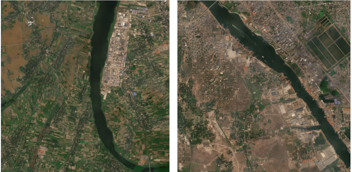
Figure 3: Representative Gamma S2DR4 2-m satellite tiles obtained after Sentinel-2 processing and super-resolution conversion. The example illustrates the high-resolution optical inputs assembled for subsequent mosaicking and LULC inference.
