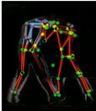
Figure 4.4: Sample Output Frame from Frame Difference on MoveNet Preprocessing
