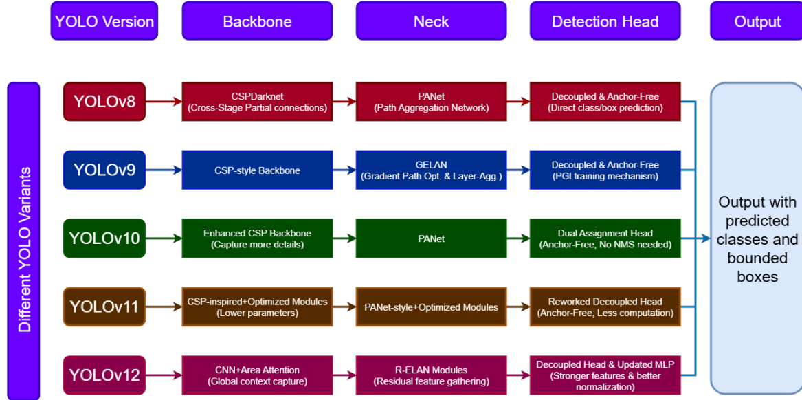
Figure 4.4: Comparative summary of the latest YOLO-based object detection models in this study
