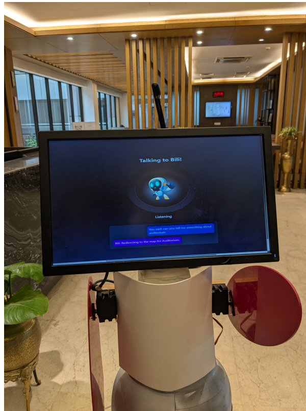
Figure 5.19: Head module with 15-inch HD display and embedded sensory components.
