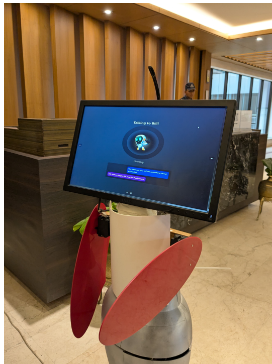
Figure 5.23: Side view showing BILI's base, torso, and head modules.
