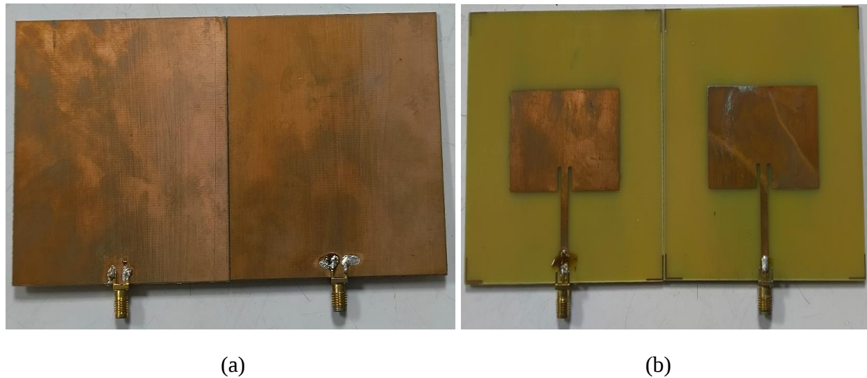
Fig 4.3. Fabricated assembled patch antenna (a) upward side and (b) downward side
