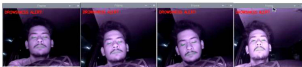
Figure 9: RPI Detecting Driver's Drowsiness
