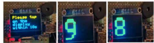
Figure 16: 10 Sec Countdown Alert Message Displayed on The Wristband's Display
