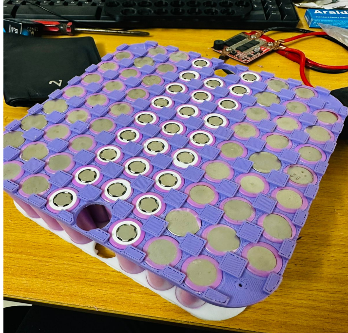
Fig.6.7: A single layer of MotorX's battery pack
