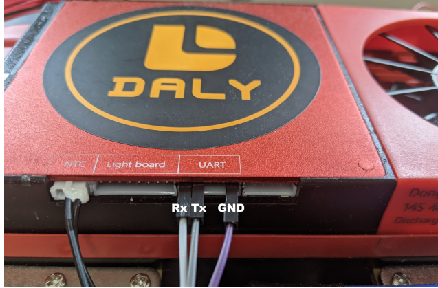
Fig 5.6 Daly BMS UART Communication with Esp32
