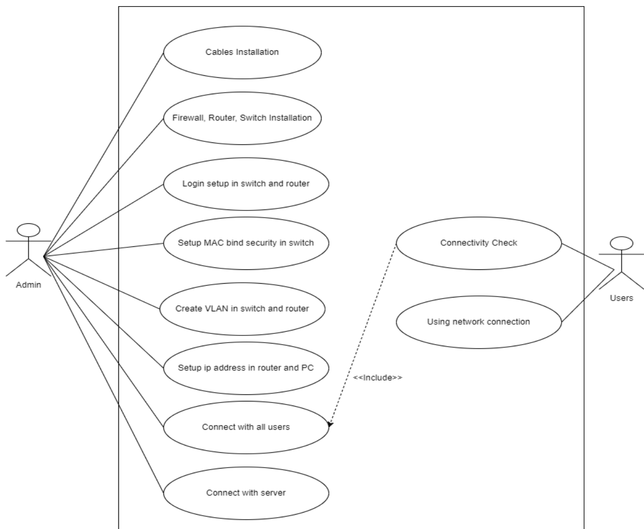
Fig 5.3.1a : Use case diagram for infrastructure design
