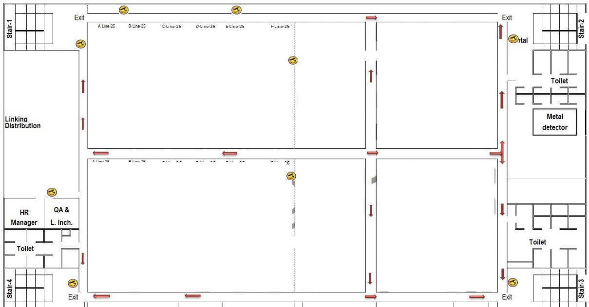
Figure 11: CCTV layout for DEPZ Factory Third Floor
