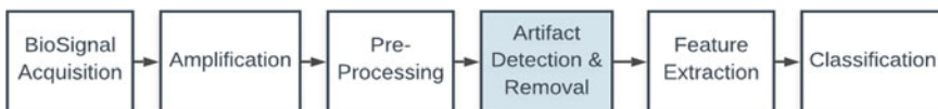
Fig. 2.1 Typical process flow of a biosignal processing system. Only artifact detection and removal is covered in this chapter
