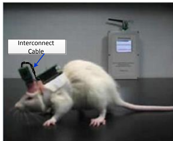
Figure 1.1: A typical experimental set-up for in-vivo extracellular neural recording of spontaneous neural activity from a freely moving subject.
